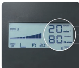
Stability can be checked with the displayed torque and rotation speed
